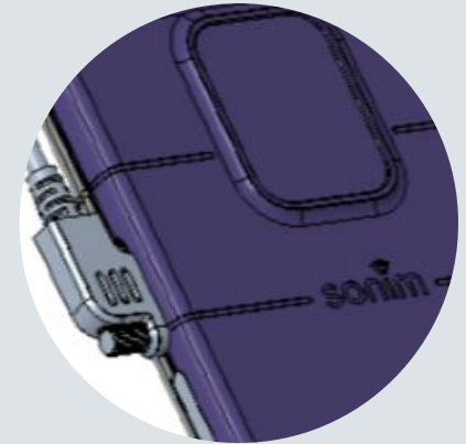
SecureAudio provides secure connection and power to accessories
